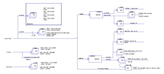
*Mezzanine supply* changes from 4v to 5v and is connected directly to the external +5v linear power supply.
