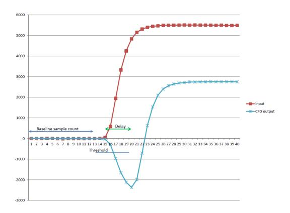
This plot shows an input waveform and a 'cfd\_output' as calculated by Excel.
