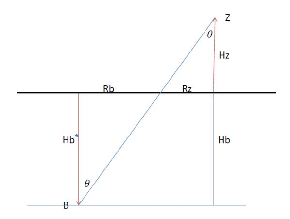
Consider the two triangles formed by the zero crossing. Assume the line joining the two points B(before Zero ) and Z ( after Zero ) is straight.
