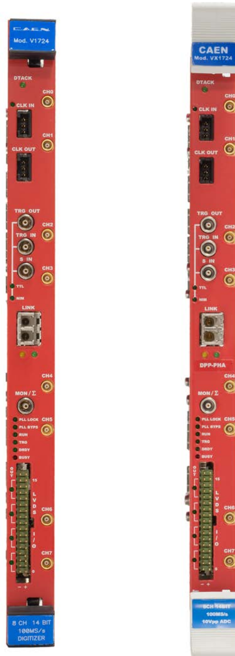
Fig. 6.1: Front panels view: V1724 on the left, VX1724 on the right
