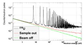
Data from a capture cross section measurement on 238U performed at the n\_TOF facility.
