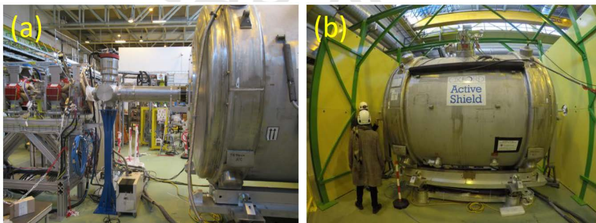
Figure 1 Photographs of the ISS magnet (a) on its base frame and connected to the beam line and (b) inside the magnetic shielding.
