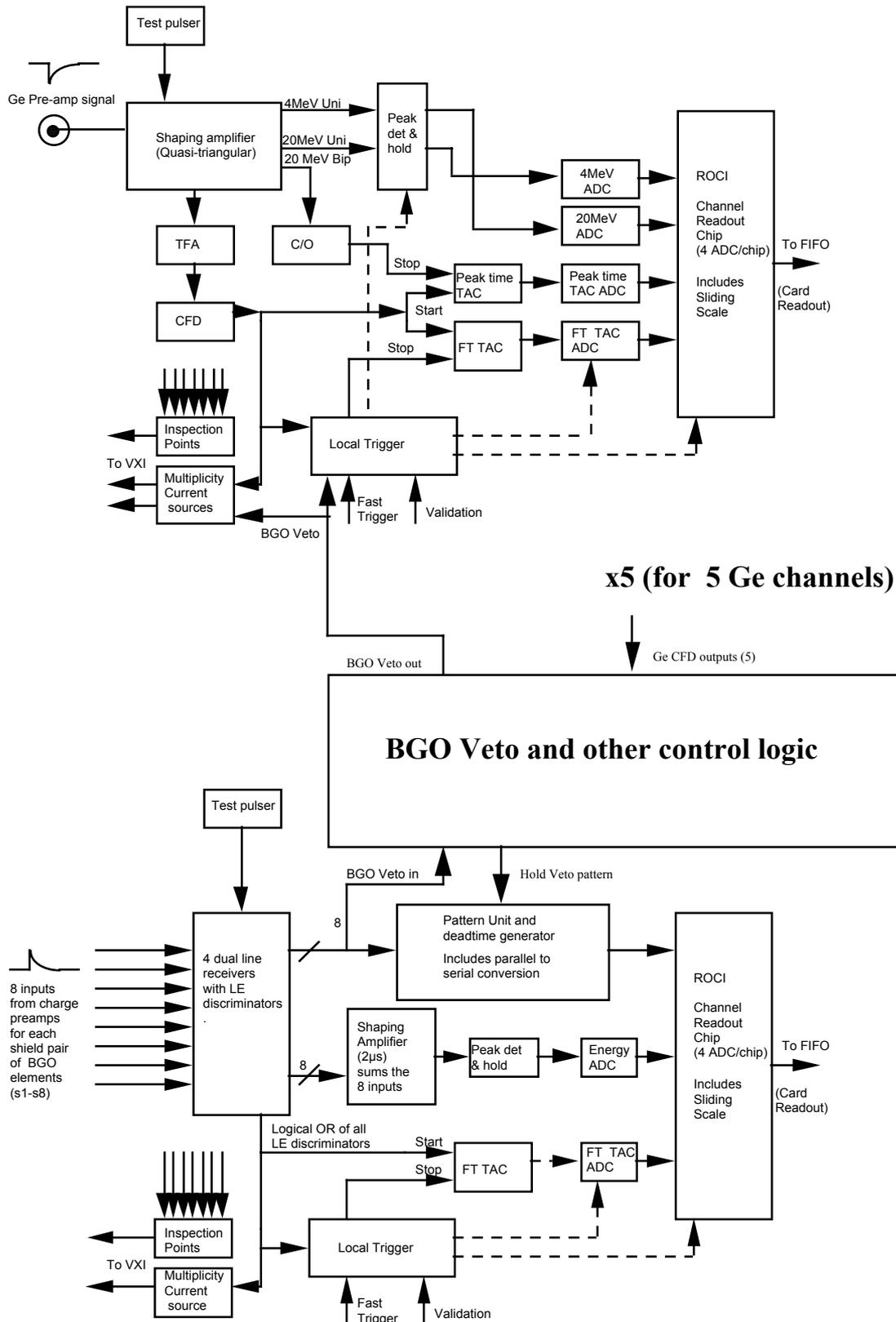
**Fig 1 Block diagram of Eurogam Phase 2 Detector Card**
