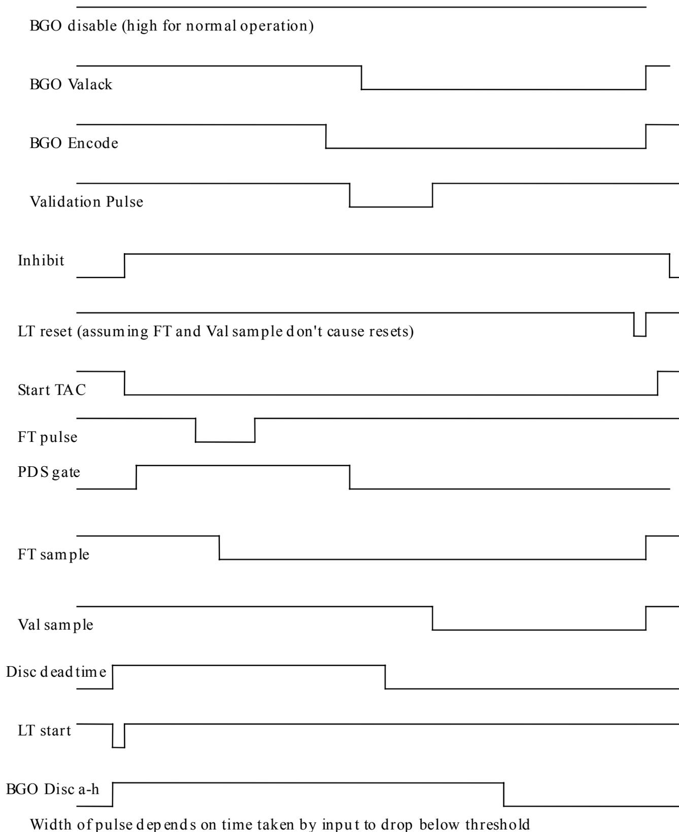
**fig 10 BGO logic inspection lines**
