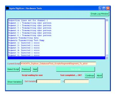
Select and run the *Segment\_init.tcl* script which checks communication with the segment module using a bit test with register 2 and changes the state of LED 7.
