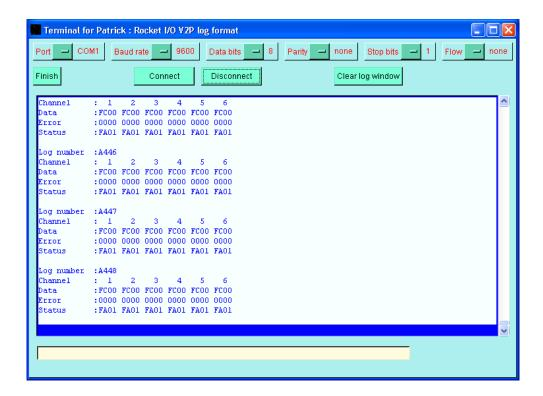
This test uses only Channel 1 of the optical receiver. The data and status reposrting is only relevant for this channel. The error counter has no meaning for this test.
