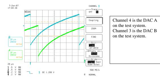
Press "continue" to insert an error into each of the channels in turn. Check only 1 error is seen at the receiver for each channel in turn. One error is reported at the start of the test as the receiver picks up the place in the ramp.
