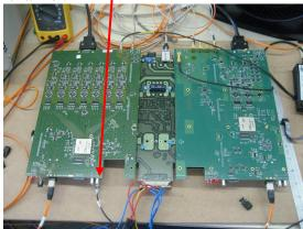
Connect the pulse signal to the analogue input on the Segment test board and run the Segment\_Digital\_Inspection.tcl script. Step through the analog and digital inspection signals checking the 'scope output for each one. The script also switches the Gain setting for each channel.
