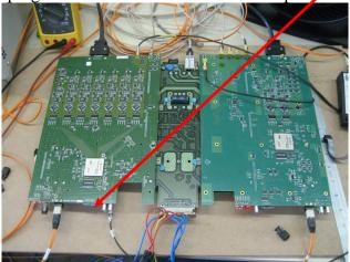
Open Impact (Xilinx programming software) and launch the wizard to check the JTAG chain. In Impact open the Segment.ipf file to setup the programming environment.
