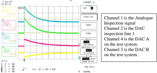
Press "Continue" to transmit the test ramp on all six channels, check the scope for channel 1 and 2 data from the test system DACs and the terminal for changing data on all six channels. The status words should all remain stable. That is they should report 0x#000 where the # nibble is allowed to change.
