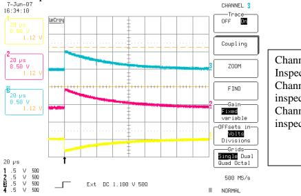
Channel 1 is the Analogue Inspection signal Channel 2 is the DAC inspection line 1 Channel 3 is the DAC inspection line 2
