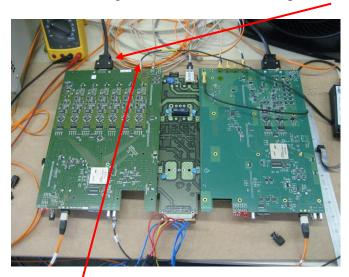
Connect the Analogue inspection signal to a 'scope with source pulse input to a second channel.
